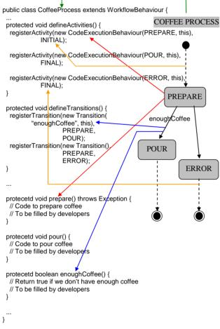
Figure 6. Workflow class structure
