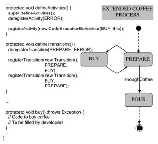
Figure 7. Workflow inheritance example
