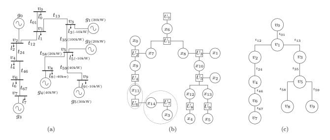
Figure 1: (a) An electricity distribution network. Showing example values for generator's maximum output, distribution cable's thermal capacity and power consumption at the loads. Node  $v_0$  is connected to the rest of the electricity grid. (b) A factor graph representation of the same network. (c) The tree representation used by DYDOP.
