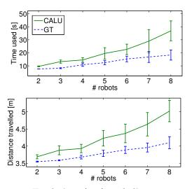
Figure 5: Total time (top) and distance travelled (bottom) metric for CALU and ground truth (GT) averaged over 50 simulations runs.
