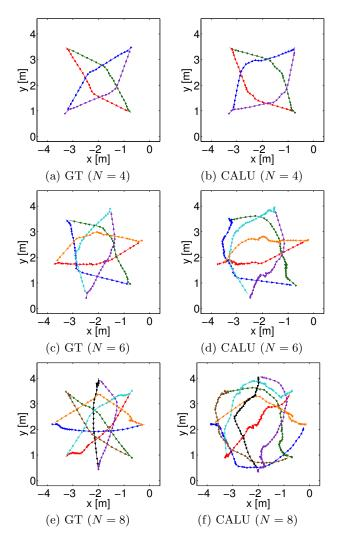
Figure 4: Typical robot trajectories observed for different numbers of robots when comparing ground truth (GT) to CALU.
