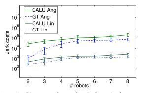
Figure 6: Linear and angular jerk costs for ground truth (GT) and CALU averaged over 50 simulation runs.
