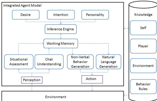
Figure 2: A schematic of the integrated agent model.
