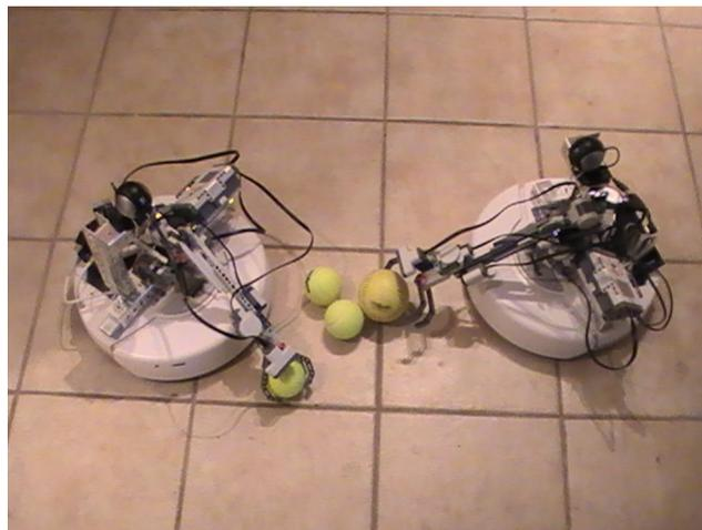
**Figure 1: Two HU-IE robots cooperating together to clear the environment of objects and deposit them in the goal location.**
