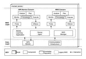
Figure 3: Example instance of SA-MAS architecture
