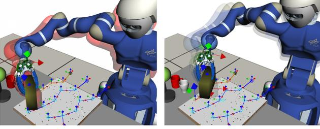
**Figure 8:** Initially, each node is directed towards the next node in the graph. If this pose is in collision (left), or unreachable, e.g. due to joint limitations (right), the free DOF of the tool are exploited.
