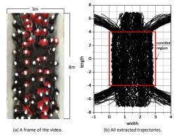
Figure 1: Corridor dataset. (a) A frame of the video; (b) All extracted trajectories in this scenario.
