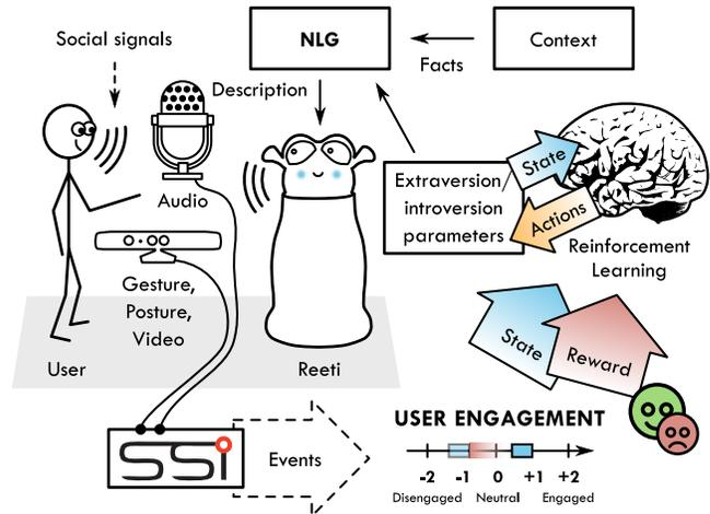
Figure 3: Manipulating robot extraversion based on social signals and RL.
