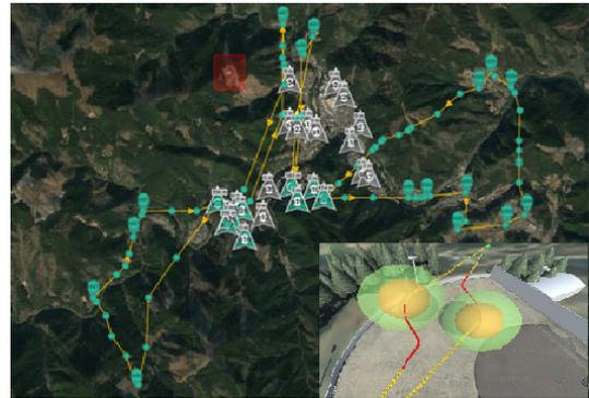
**Figure 1: Example of task allocation for one UASSP and example of Adapted ORCA solving a conflict between 2 UAVs. The different safety layers spheres around each UAV are represented in yellow and green. Paths modified by Adapted ORCA are represented in red.**
