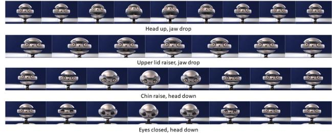
**Figure 1: Robot expressions: Head up, jaw drop (HU-JD); Upper lid raiser, jaw drop (ULR-JD); Chin raise, head down (CR-HD); Eyes closed, head down (EC-HD). Note: these acronyms are used henceforth.**
