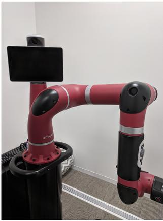
Figure 2: Sawyer robot has seven degrees of freedom.
