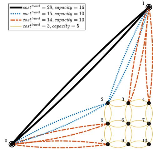
**Figure 3: The basic traffic graph.** AGVs are initialized at 0 and 1, traveling to the opposite vertex, i.e. vertex 1 or vertex 0, respectively. Edges (0, 1), and (1, 0) have the highest capacity and represent the shortest path. The goal of the multiagent traffic management team is to incentivize detours to alleviate congestion. Figure from [4].
