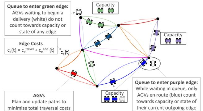
**Figure 1: The environment is described by a traffic graph where each directed edge must obey strict capacity constraints. AGVs cannot enter edges that are already at capacity. Those waiting to transition between edges continue to occupy space on their current edge. The goal of the traffic management domain is to find the set of additional cost functions  $c_e^{add}(t)$  that result in the maximal number of successful deliveries.**
