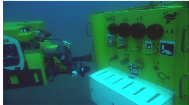
Figure 1: ROV performing oil & gas valve manipulation.
