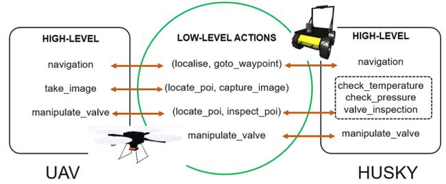
**Figure 2: Mapping from an H-L action for a husky and UAV to a sequence of L-L actions. More than one H-L action can be mapped to an L-L action using different grounding.**
