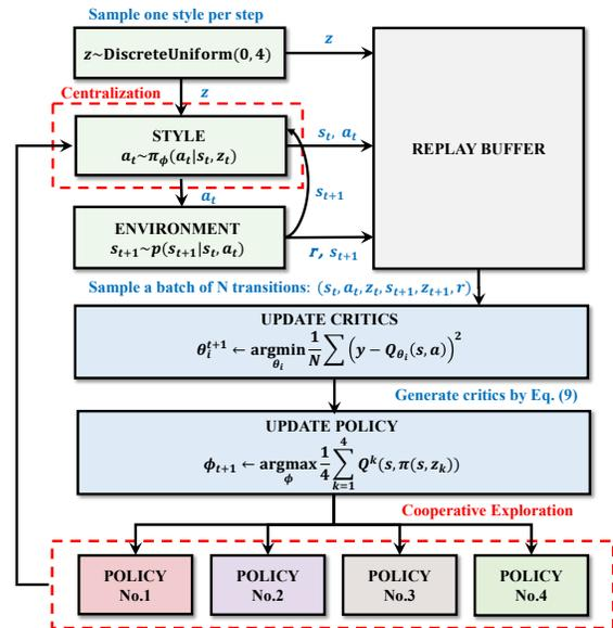
Figure 1: The workflow of CCEP Algorithm. The agent  $\pi$  interacts with the environment with diverse style cooperatively. A centralized policy with four different styles is learned from the multi-styled critics.
