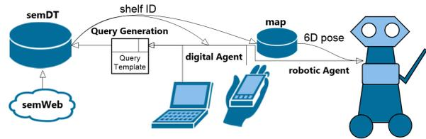
Figure 3: The Architecture of the Smartphone- and robot setup
