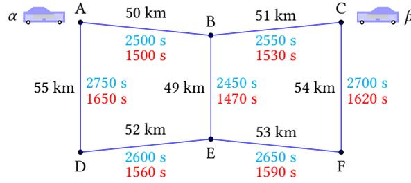
**Figure 1: Example of CEVPP where the EV  $\alpha$  must move from A to F and the EV  $\beta$  must move from C to D. Each node represent a charging station. We assume the battery of each EV is 12 kWh and the consumption is 200 Wh/km (i.e., their range is 60km). We also assume their speed is constant at 72 km/h and the charging stations have 24 kW power. The numbers in blue represent the travel time, and the numbers in red represent the corresponding charging time.**
